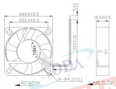
LEAD WIRES: UL 1007, AWG26, L = 300 +/- 10 mm Red = positive; Black = negative.
