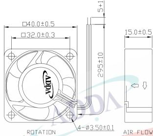
LEAD WIRES: UL 1007, AWG26, L = 295 ± 10 mm
