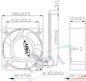
LEAD WIRES: UL 1007, AWG26, L =  $295 \pm 10$  mm Red = positive; Black = negative.
