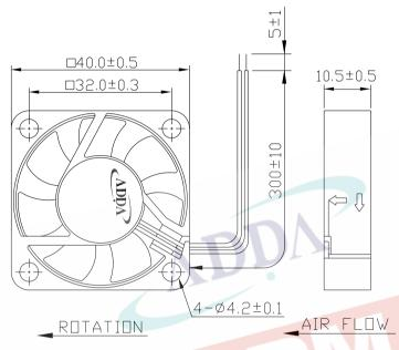
LEAD WIRES: UL 1007, AWG26, L =  $300 \pm 10 \text{ mm}$ Red = positive; Black = negative.
