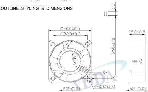
LEAD WIRES: UL 1007, AWG26, L = 295 ± 10 mm Red = positive; Black = negative.
