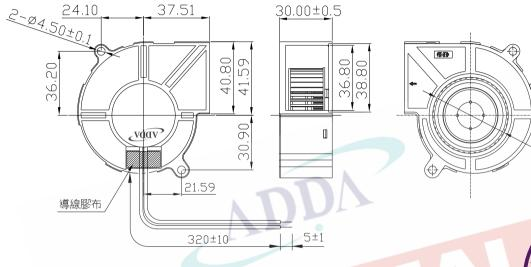
LEAD WIRES: UL 1007, AWG24, L =  $320 \pm 10$  mm Red = positive; Black = negative.
