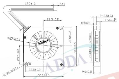
LEAD WIRES: UL 1571, AWG28, L = 120 +/- 10 mm Red = positive; Black = negative.
