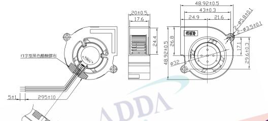
LEAD WIRES: UL 1007, AWG26, L = 295 ± 10 mm
