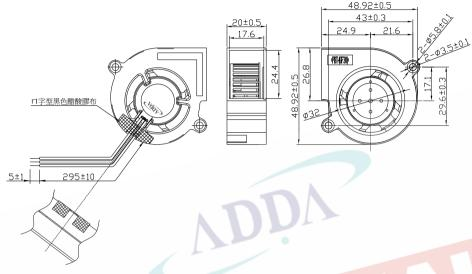
LEAD WIRES: UL 1007, AWG26, L =  $295 \pm 10$  mm Red = positive; Black = negative. White = FG
