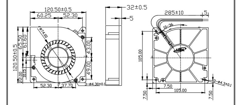
LEAD WIRES : UL 1007, AWG24 , L =  $285\pm10$  mm Red = positive ; Black = negative.
