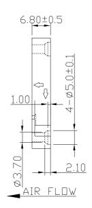
LEAD WIRES: UL 1571, AWG28, L = 135 +/- 10 mm Red = positive; Black = negative. Blue = FG
