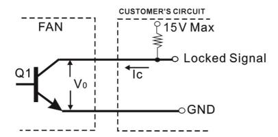
\*Transistor Q1 at "ON" position Collector current....... $I_c$ =10mA Max Saturation Voltage...... $V_{oL}$ =1.0V Max \*Transistor Q1 at "OFF" position Release Voltage...... $V_{OH}$ =15V Max
