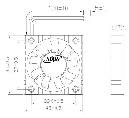
LEAD WIRES: UL 1571, AWG28, L = 130±10 mm Red = positive; Black = negative.
