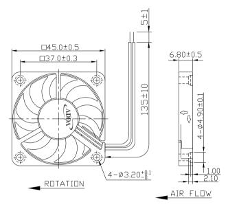
LEAD WIRES: UL 1571, AWG28, L = 135 +/- 10 mm Red = positive; Black = negative.
