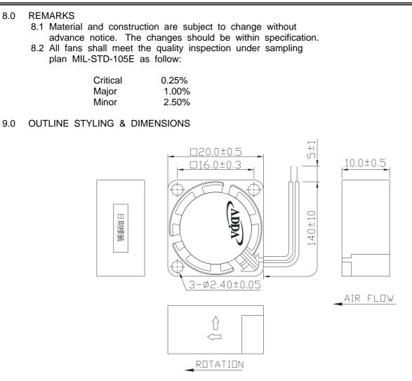
LEAD WIRES : UL 1571, AWG28 , L = 140 +/- 10 mm Red = positive ; Black = negative.
