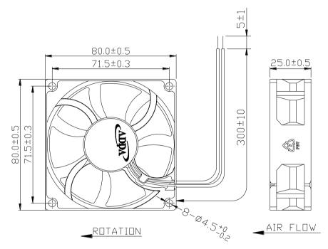
LEAD WIRES: UL 1007, AWG24, L = 300±10 mm Red = positive; Black = negative.
