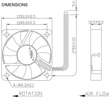
LEAD WIRES : UL 1007, AWG26 , L = 290 +/- 10 mm Red = positive; Black = negative. Blue = FG
