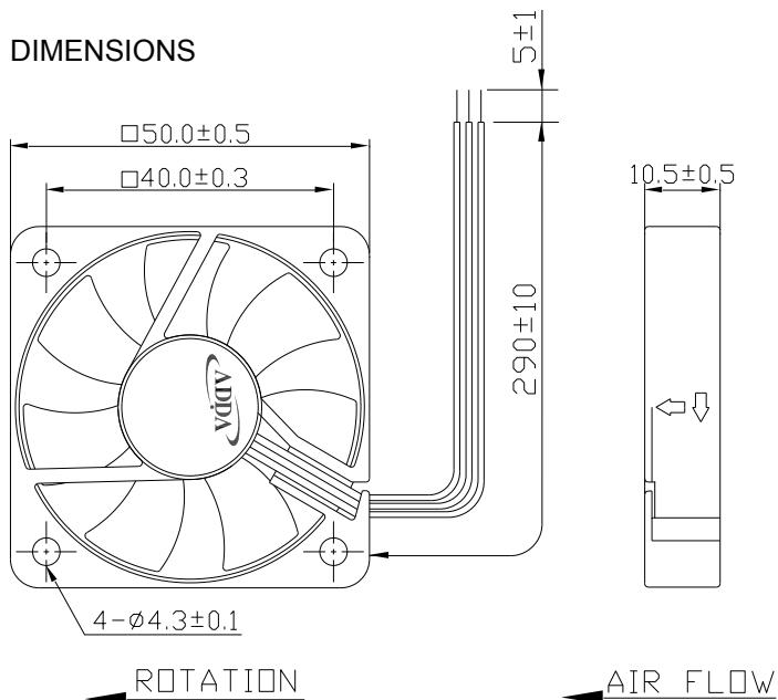
LEAD WIRES : UL 1007, AWG26 , L = 290 +/- 10 mm
