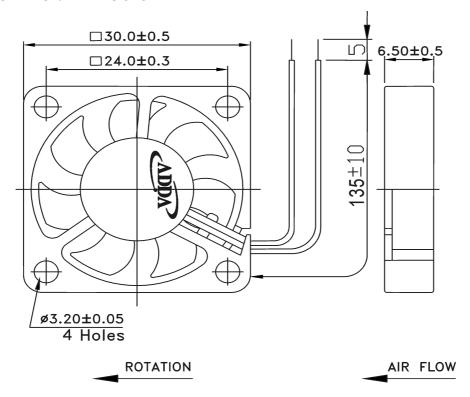
LEAD WIRES: UL 1571, AWG28, L = 135 +/- 10 mm Red = positive; Black = negative.
