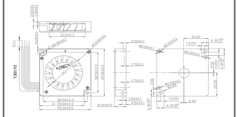
LEAD WIRES: UL 1571, AWG28, L = 130 +/- 10 mm Red = positive; Black = negative. White = FG ; Blue = pwm input
