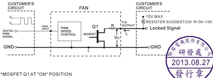
DRAIN CURRENT----------I<sub>D</sub>=5mA MAX SATURATION VOLTAGE------- V<sub>01</sub> = 1.0 V MAX
