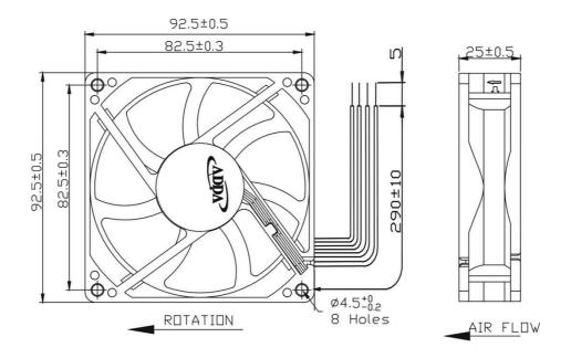
LEAD WIRES : UL 1061, AWG26 , L =  $290\pm10$  mm Red = positive ; Black = negative. White = FG : Blue = PWM
