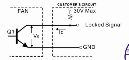
\*Transistor Q1 at "ON" position
