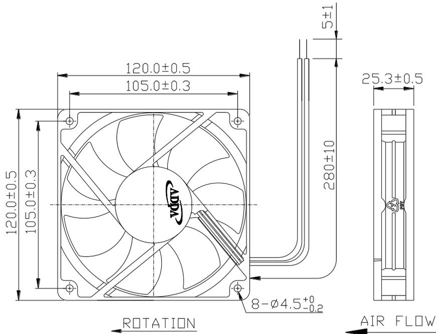
LEAD WIRES : UL 1007, AWG24 , L = 280±10 mm
