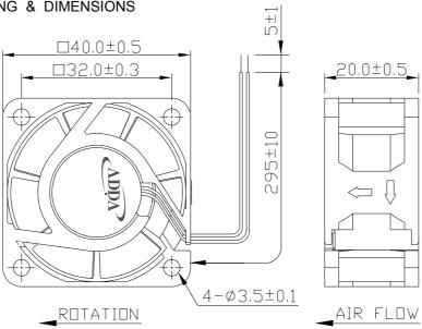
LEAD WIRES: UL 1007, AWG26, L = 295 +/- 10 mm Red = positive; Black = negative.
