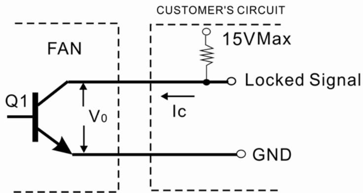
\*Transistor Q1 at "ON" position
