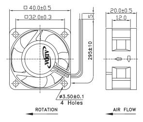
Frame:Plastic(UL:94V-0) Impeller:Plastic(UL:94V-0) Lead wire:UL1007AWG26
