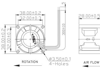
Frame:Plastic(UL:94V-0) Impeller:Plastic(UL:94V-0) Bearing:Ball bearing Lead wire:UL1061AWG26 VOLTAGE AVAILABLE:12V
