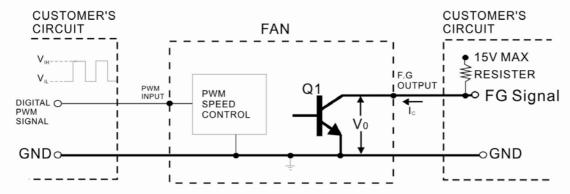
\*TRANSISTOR Q1 AT "ON" POSITION
