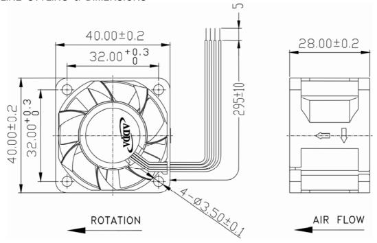
LEAD WIRES: UL 1061, AWG26, L = 295 +/- 10 mm Red = positive; Black = negative. White = FG; Blue = pwm input
