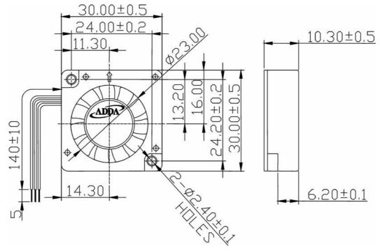
LEAD WIRES : UL 1571, AWG28, L = 140 +/- 10  $\,$  mm Red = positive ; Black = negative.
