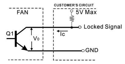
\*Transistor Q1 at "ON" position
