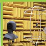
Semi-anechoic chamber According ISO 3744 According ISO 3745 According ISO 7779
