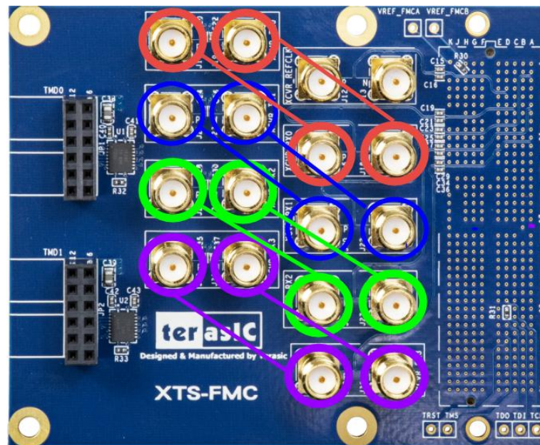
Figure 4-1 SMA loopback setup
