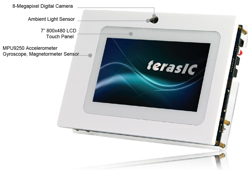
Figure 2-1 VEEK-MT2 PCB and Component Diagram (top view)
