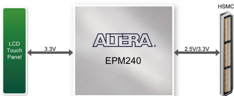
Figure 3-6 Block Diagram of the Bus Controller
