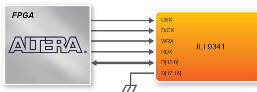
Figure 3-2 Signals of LCD driver connected to FPGA
