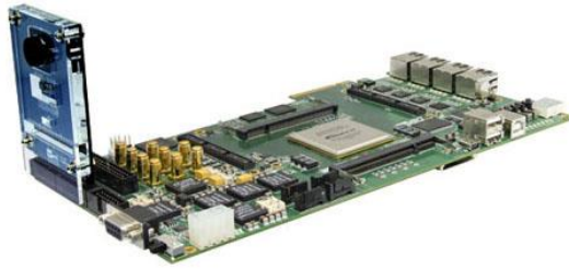
Figure 1-2 Connect the D5M to DE4 board's expansion port (outermost port).
