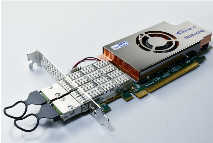
Figure 7-4 Two QSFP+ Loopback Fixtures Installed
