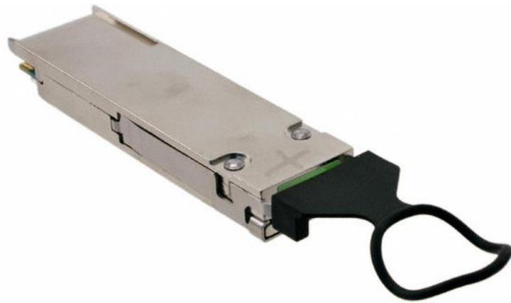
Figure 7-2 QSFP+ Loopback Fixture
