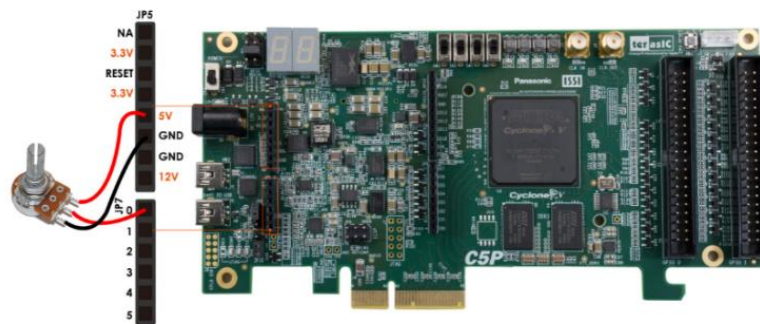
Figure 5-20 ADC Reading Demo hardware setup
