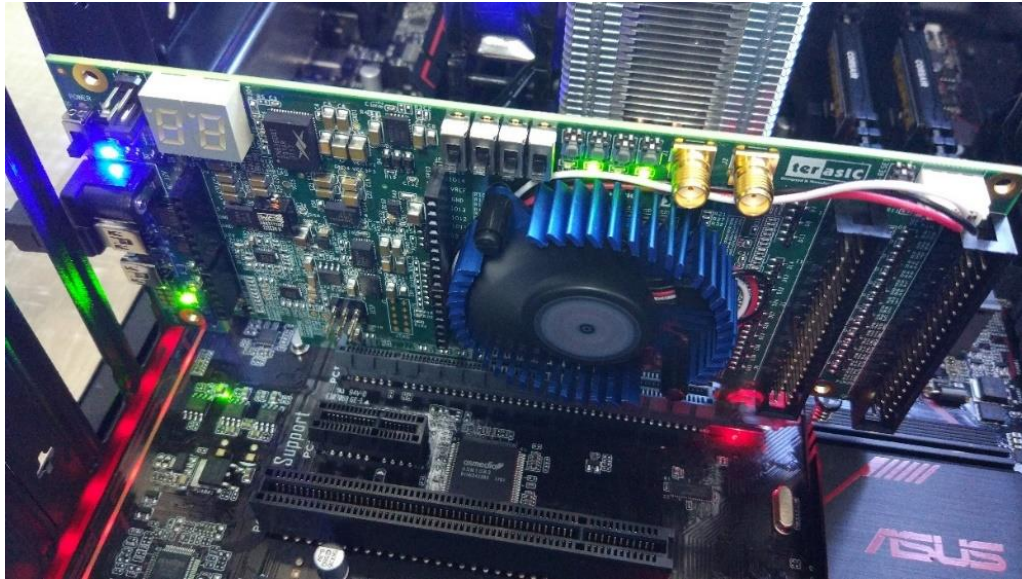
Figure 7-3 Install the FPGA board on the PC
