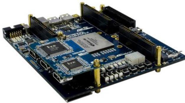
Figure 1-2 Connect HDMI daughter board to DE3 board
