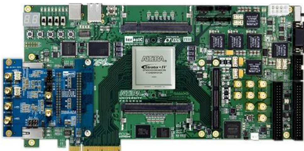
Figure 1-6 Connect ADA-HSMC with DE4 (HSMC port A)
