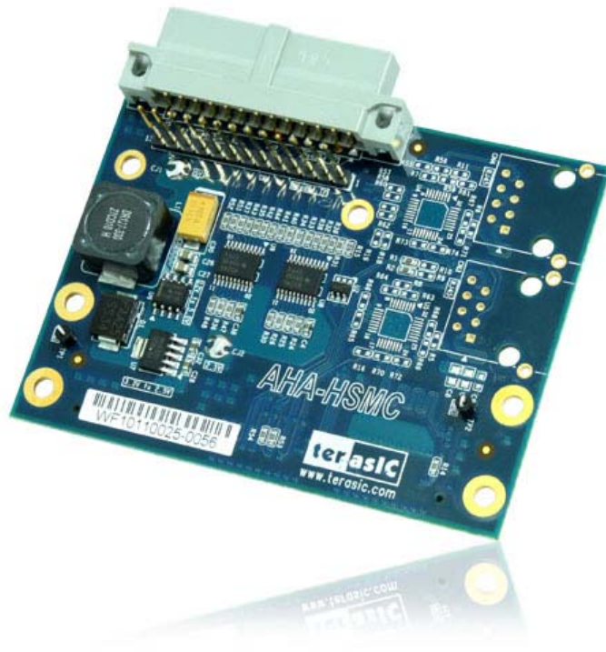
Figure 1-1 Layout of the AHA-HSMC card
