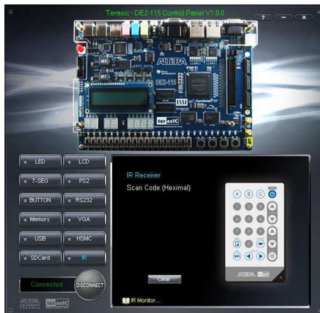
Figure 3-14 Testing the IR receiver using remote controller
