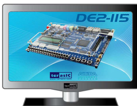
Figure 2-4 The default VGA output pattern
