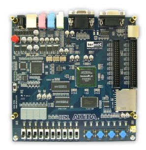
audio applications and video. Finally, it is possible to connect other user defined boards to the DE1 board by means of two expansion headers.
