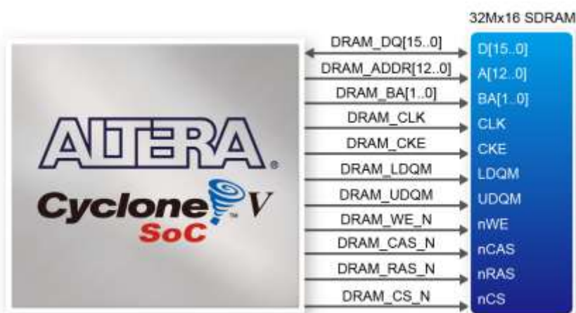
Figure 3-28 Connections between the FPGA and SDRAM
