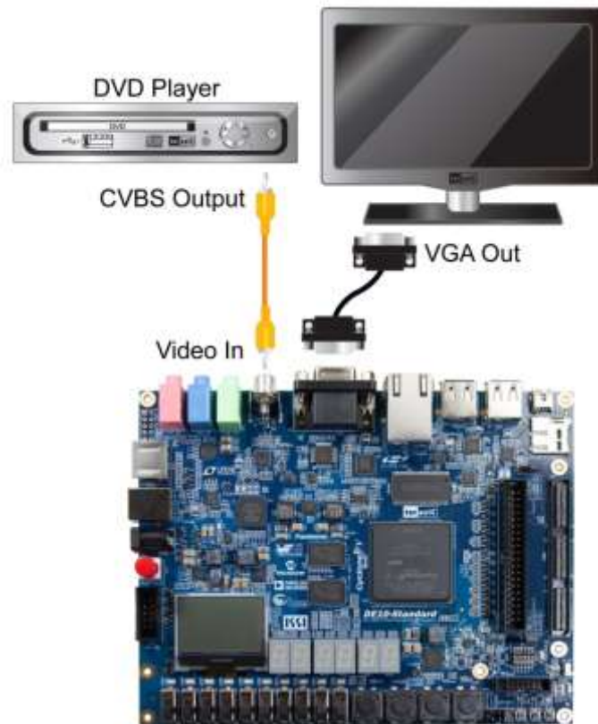
Figure 5-12 Setup for the TV box demonstration (VIP)
