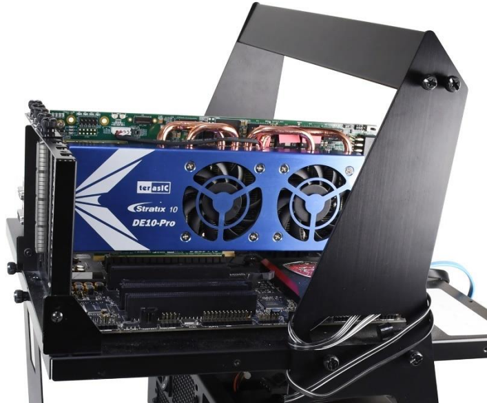
Figure 7-9 FPGA board installation on PC
