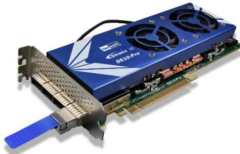
Figure 9-7 Setup QSFP28 loopback fixture
