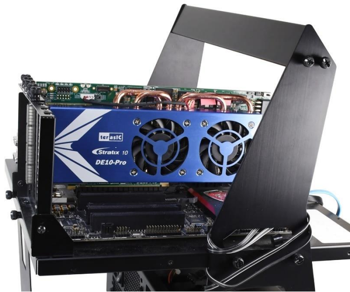
Figure 8-4 FPGA board installation on PC
