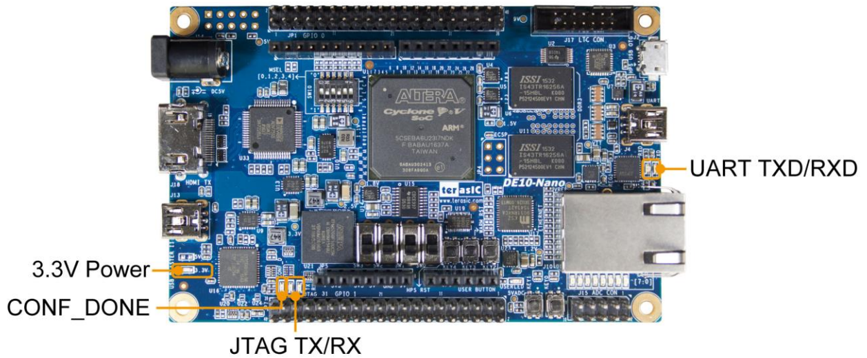
Figure 3-12 LED Indicators on DE10-Nano
