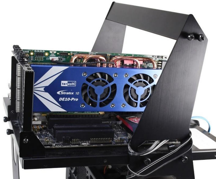
Figure 7-9 FPGA board installation on PC
