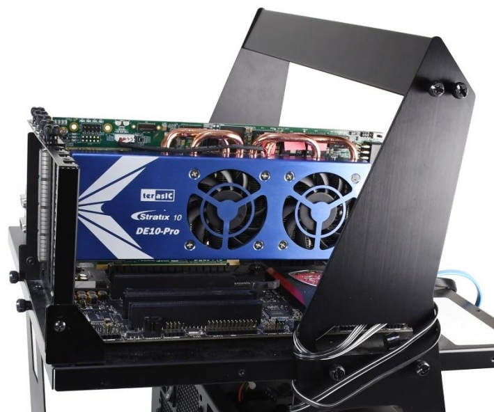
Figure 8-4 FPGA board installation on PC
