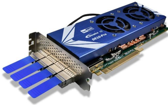
Figure 9-2 QSFP28 Transceiver Loopback Test in Progress
