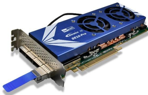
Figure 9-7 Setup QSFP28 loopback fixture
