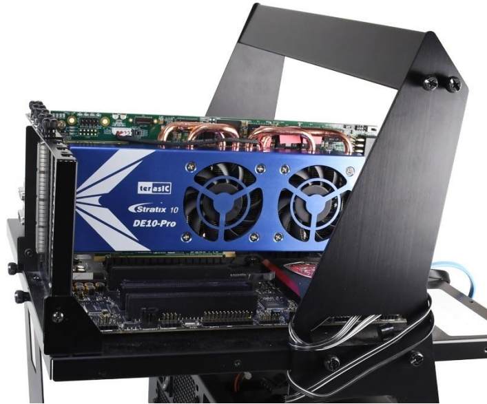
Figure 7-9 FPGA board installation on PC
