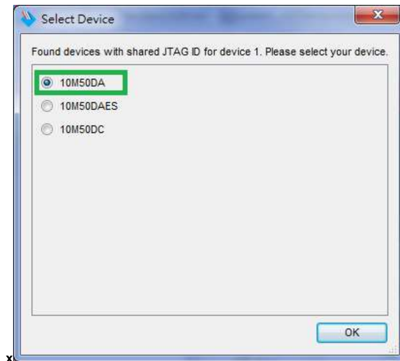
Figure 3-5 Select 10M50DA device
