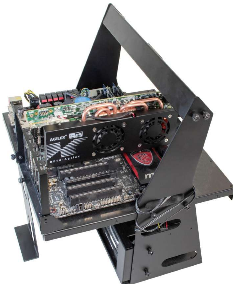
Figure 7-9 FPGA board installation on PC
