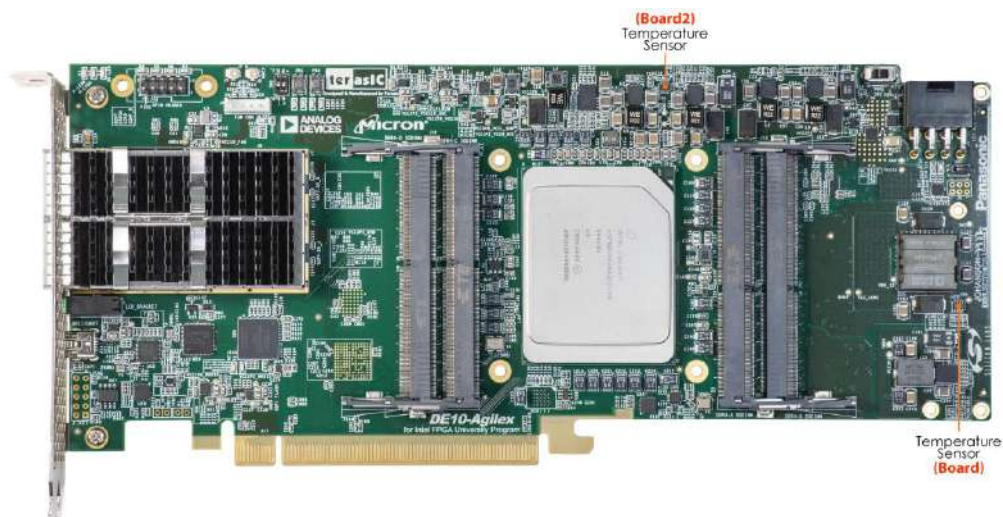
Figure 10-10 Location of the board's ambient temperature
