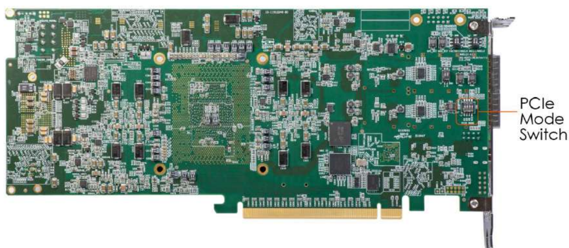
Figure 2-7 Position of the PCIe mode switch
