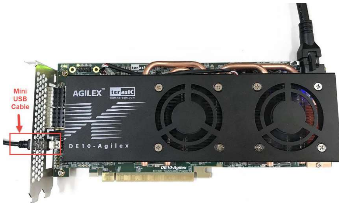
Figure 10-2 Connection setup for using dashboard system
