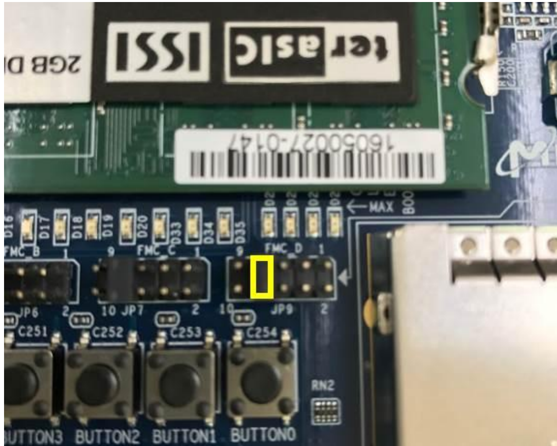
Figure 4-4 Adjust FMC_D VADJ to 2.5V by short JP9.7 and JP9.8
