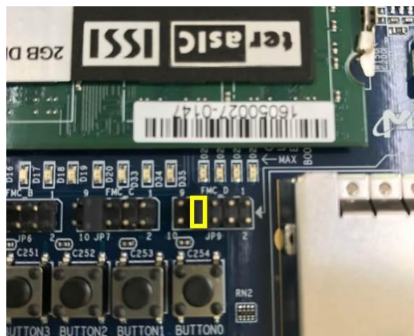
Figure 5-6 Adjust FMC_D VADJ to 2.5V by short JP9.7 and JP9.8
