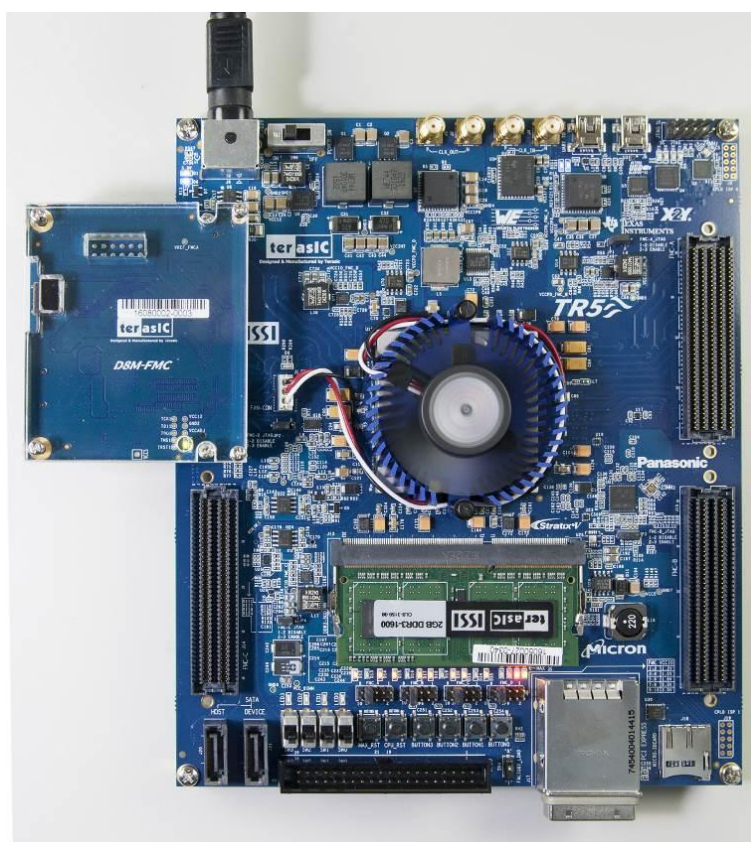
Figure 1-2 Connect the D8M-FMC to TR5 board's expansion port
