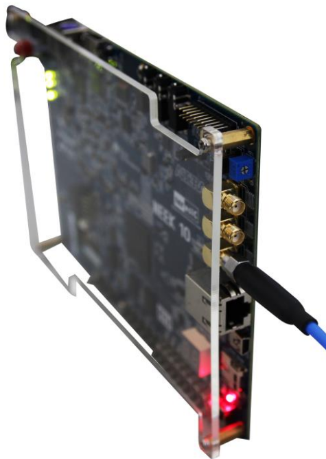
Figure 5-7 Probe DAC SMA OUT from the Oscilloscope
