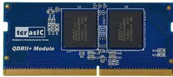
Figure 4-18 Terasic QDR II+ module with DDR4 SO-DIMM interface
