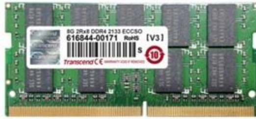
Figure 4-17 Standard DDR4 SO-DIMM with ECC
